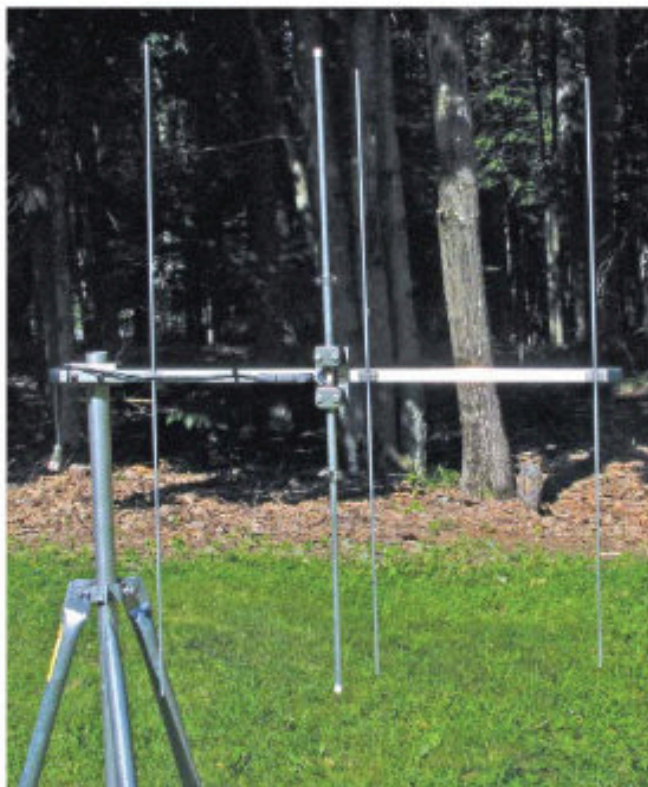
The 2-meter Yagi mounted in the vertical polarization. [Joe Reisert, W1JR, photo]
